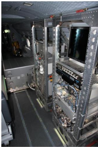
Figure 3: Photograph of the CO 2 and CH 4 IPDA lidar as installed into the cabin of HALO.
