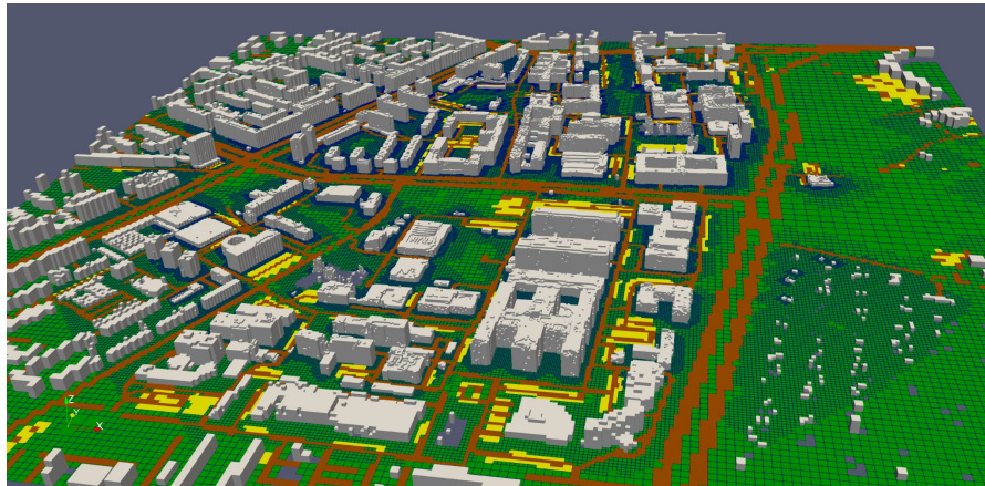
Fig.: Example of mesh generated for area 1x1km in Warsaw
