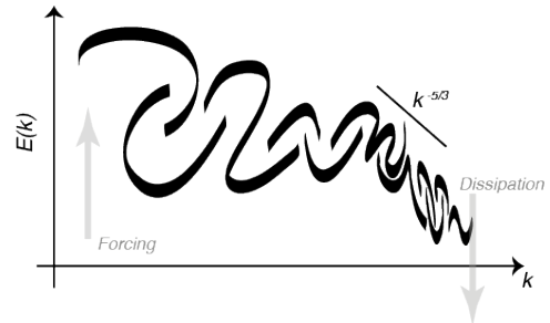
Figure 2.11 Cartoon of energy cascade whereby energy “cascades” inviscidly from large scales to small scales where it is then dissipated. Here the scale of the motion is denoted by its wavenumber k = 2\pi/l where l is the wavelength.
