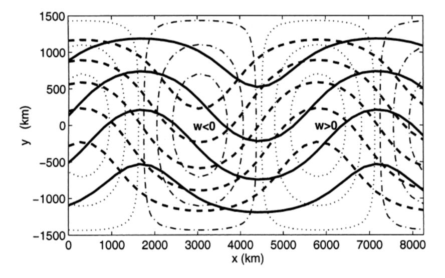
Schematic 500-hPa height contours (solid lines), isotherms (dashed lines), and vertical motion field (w > 0 dash-dot lines, w < 0 dotted lines) for a developing synoptic-scale system. Upward motion occurs where vorticity decreases moving left to right along an isotherm, and downward motion occurs where vorticity decreases moving left to right along an isotherm.
