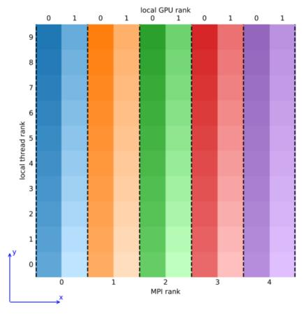
Top-down view of modeled domain; squares are Eulerian grid cells; coloring shows MPI, thread and GPU ranks.
