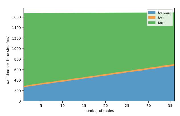
Wall time per time step vs number of nodes. Timings of simultaneous CPU and GPU computations (blue), CPU-only computations (orange) and GPU-only computations (green) are stacked.
