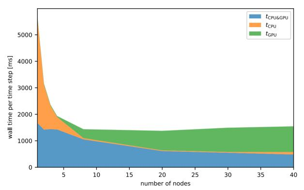
Good balance of CPU and GPU computations (ca. 80%) for an optimal number of nodes (5-10 in this case)
