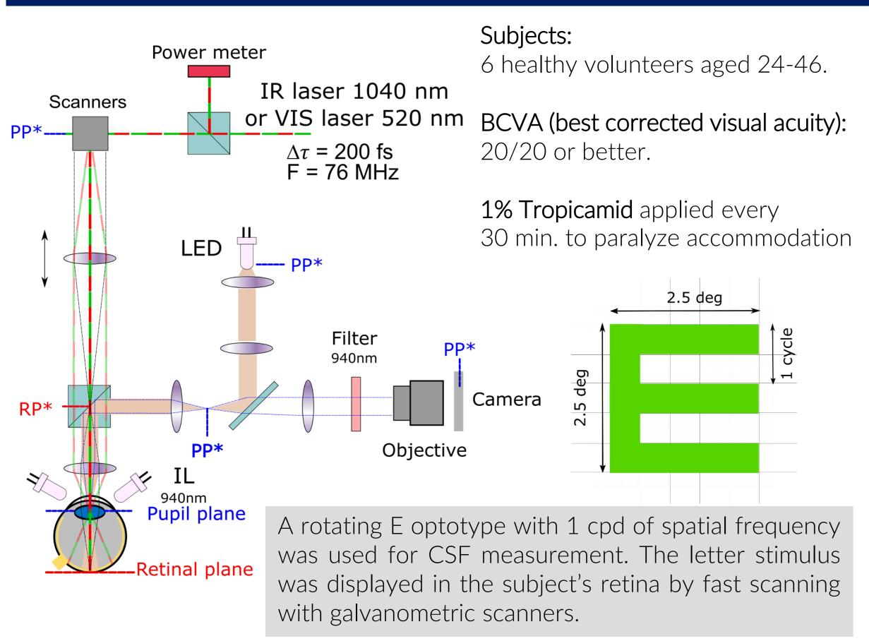
Fig 1. Optical system. The IR and VIS beams were generated by a femtosecond laser (=200 fs, Frep=76 Hz). BS, beam splitter; CAM, camera; DM, dichroic mirror; GS, galvanometer scanners; IF, 940 nm bandpass filter; Li, lens; LED, white LED; OBJ, objective; PM, power meter; PP, pupil plane; PP\*, conjugated pupil plane; RP, retinal plane; RP\*, conjugated retinal plane.
