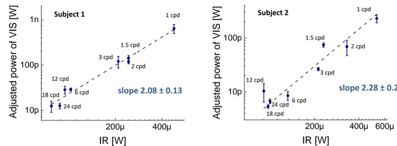
**Fig 2.** The adjustment relationship of the visible beam power, corresponding to the brightness of the stimulus with a specific infrared beam power. The quadratic relationship of the adjusted visible beam power to the infrared beam power emphasizes the nonlinear character of the two-photon vision.
