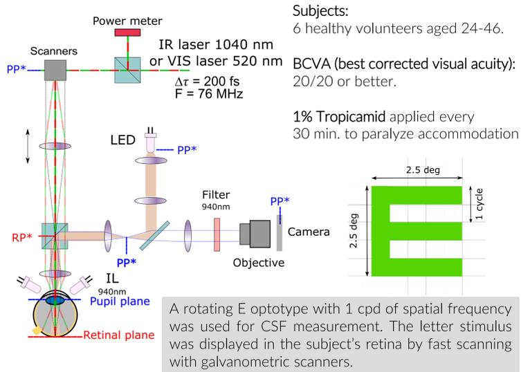
**Fig 1.** Optical system. The IR and VIS beams were generated by a femtosecond laser (=200 fs, Frep=76 Hz). BS, beam splitter; CAM, camera; DM, dichroic mirror; GS, galvanometer scanners; IF, 940 nm bandpass filter; Li, lens; LED, white LED; OBJ, objective; PM, power meter; PP, pupil plane; PP\*, conjugated pupil plane; RP, retinal plane; RP\*, conjugated retinal plane.
