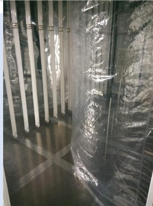
ACD-C smog chamber
