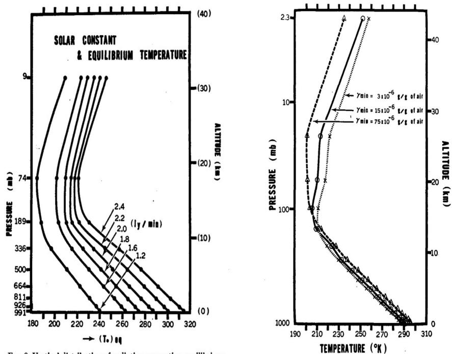
FIG. 8. Vertical distribution of radiative convective equilibrium temperature of the atmosphere with a given distribution of relative humidity for various values of the solar constant.
