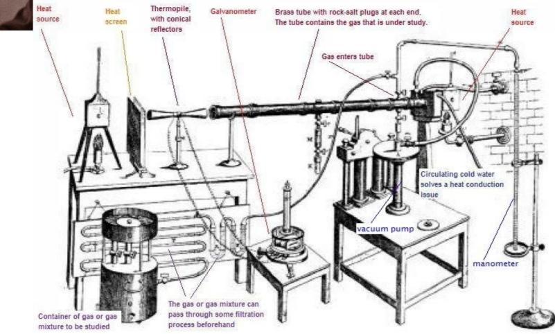
1861, Tyndall's apparatus measuring properties of greenhouse gases.
